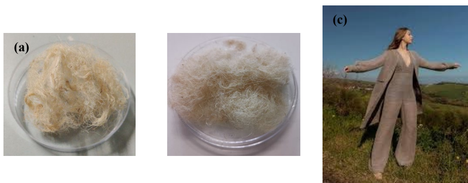
Figure 1: Representative samples of the raw (a) and treated cellulose fiber with the chemical softener (b). Prototypes of dresses for women, a trench coat and a jumpsuit, with broom and linen fibers (c).
